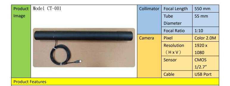
• Set 1" to 100"/grid the scale value of the electronic reticle  $\rightarrow$  Highly increased measurement
